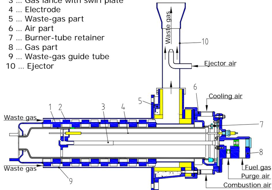
The **burner** is comprised of a three-part burner head, recuperator as well as such components as burner tube, gas lance, and electrode installed inside.
