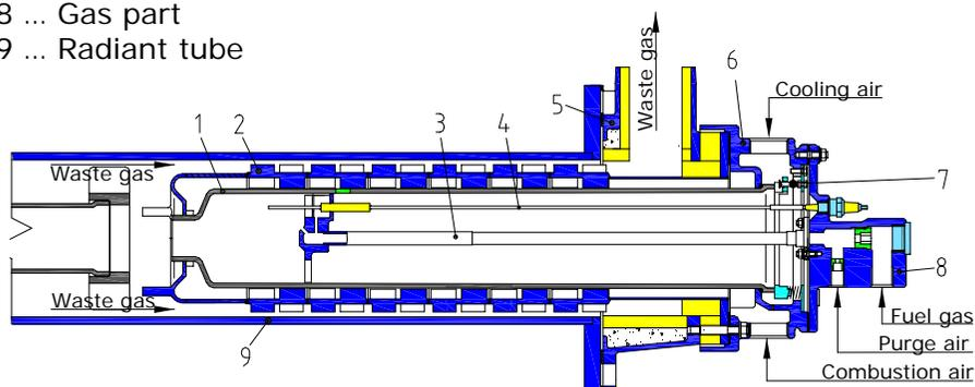
The **burner** is comprised of a three-part burner head, recuperator as well as such components as burner tube, gas lance, and electrode installed inside. The burner is suited both for horizontal and vertical installation.
